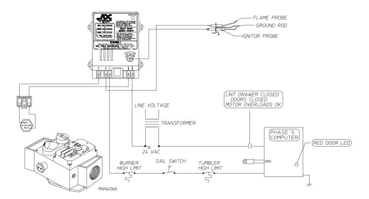
a. The Direct Spark Ignition (DSI) Module is a 24 VAC device designed to be the "controller" of the DSI system. When activated by the dryer controls, this module constantly monitors and controls the functions of the DSI system (i.e., spark activation, gas valve off/on, flame verification, etc.). Additionally, the DSI Module has self diagnostic capabilities.
