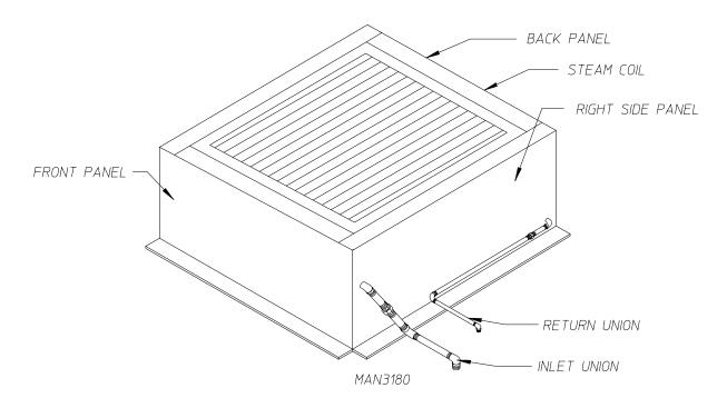
VIEW OF STEAM COIL W/ DAMPER REMOVED
