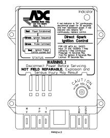
24 VAC Direct Spark Ignition (DSI) Module
