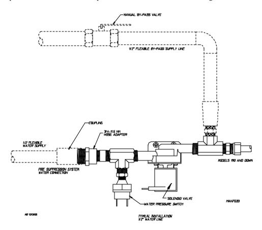
**WARNING:** If the water in the supply line or water solenoid valve freezes, the S.A.F.E. system <u>will</u> **be** INOPERATIVE!!
