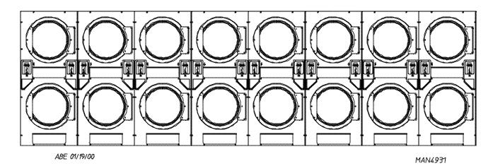
TYPICAL INSTALLATION SHOWING MAKE-UP AIR OPENINGS
