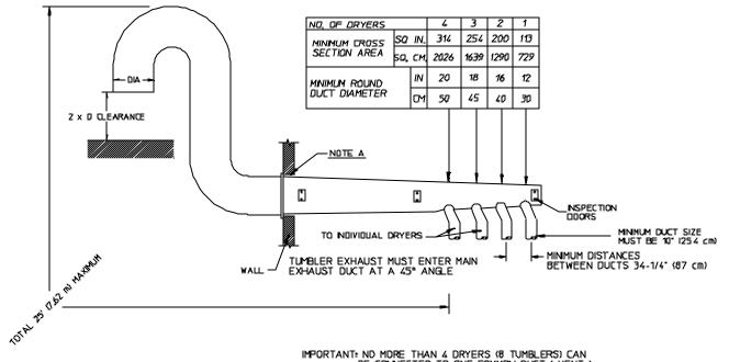
IMPORTANT: ND MORE THAN 4 DRYERS (8 TUMBLERS) CAN BE CONNECTED TO ONE COMMON DUCT ( VENT ),
