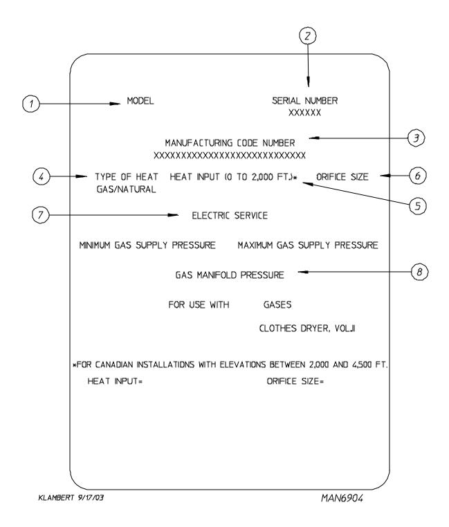
When contacting **American Dryer Corporation**, certain information is required to ensure proper service/parts information from **ADC**. This information is on the data label, which is affixed to the left side panel area behind the top control (access) door. When contacting **ADC**, please have the <u>model number</u> and <u>serial number</u> available.
