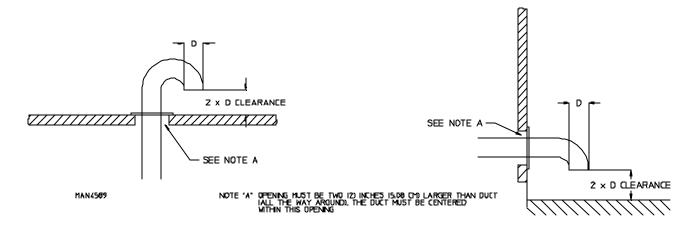
When the exhaust ductwork passes through a wall, ceiling, or roof made of combustible materials, the opening **must be** 2-inches (5.08 cm) larger than the duct (all the way around). The duct **must be** centered within this opening.
