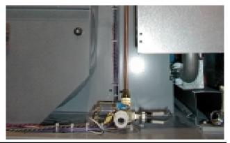
**IMPORTANT:** Flexible supply line/coupling *must be* used. Solenoid valve failure due to hard plumbing connections <u>WILL VOID WARRANTY</u>. <u>It is recommended</u> that a filter or strainer be installed in the water supply line.
