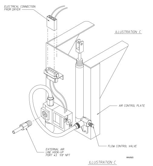
**NOTE:** Turning knob on flow control valve clockwise (CW) will restrict airflow. Turning knob on flow control valve counterclockwise (CCW) will increase airflow.
