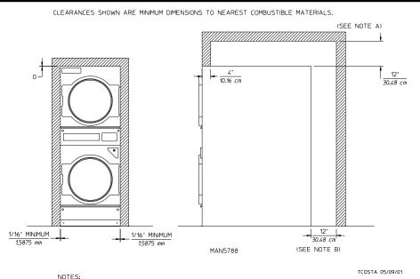
A. MINIMUM OF 12" (30.48 cm) CLEARANCE IS ACCEPTABLE FOR EASE OF INSTALLATION AND SERVICE (POWER CONNECTIONS). AT LEAST 18" (45.72 cm) IS RECOMMENDED.
