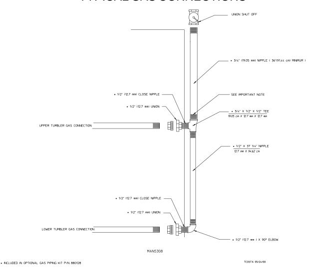
**IMPORTANT:** When plumbing upper and lower baskets (tumblers) together, as illustrated above, supply connection *must be* a minimum of 3/4" (19.05 mm).
