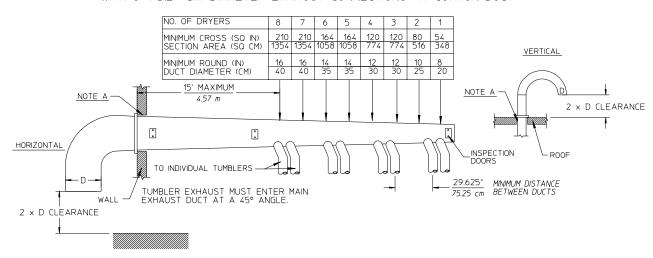
IMPORTANT: NO MORE THAN 4 DRYERS (8 TUMBLERS) CAN BE CONNECTED TO ONE COMMON DUCT (VENT).
