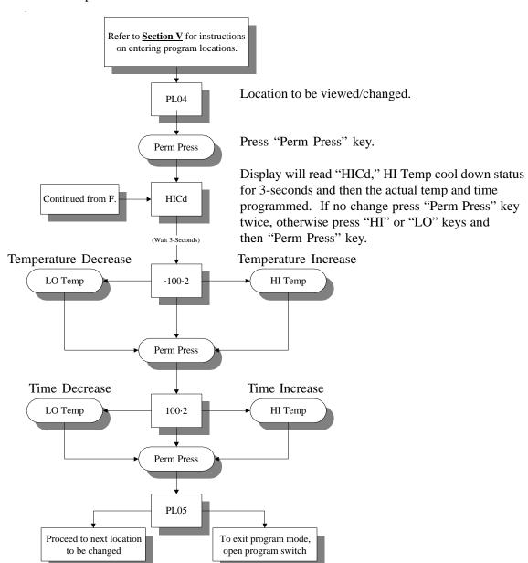
Summary: Cool down temperature is programmable from a minimum of 100° F to a maximum of 160° F in ten-degree increments or from a minimum of 38° C to a maximum of 71° C in five-degree increments.
