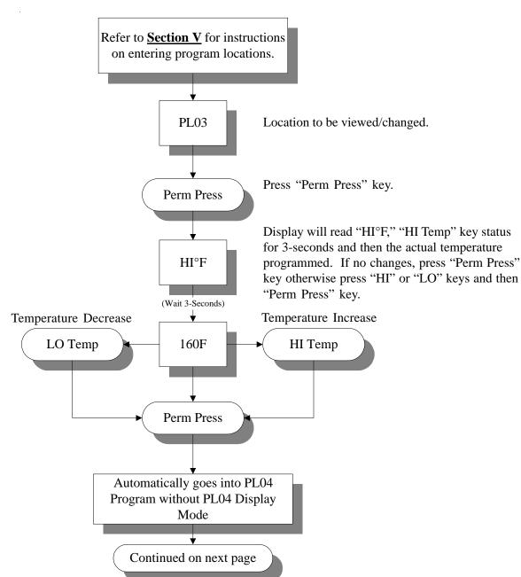
Summary: The high (HI) operating temperature is programmable from a minimum of 100° F to a maximum of 160° F in ten-degree increments or from a minimum of 38° C to a maximum of 71° C in five-degree increments.
