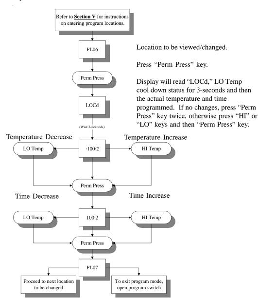
Summary: Cool down temperature is programmable from a minimum of 100° F to a maximum of 160° F in ten-degree increments or from a minimum of 38° C to a maximum of 71° C in five-degree increments.
