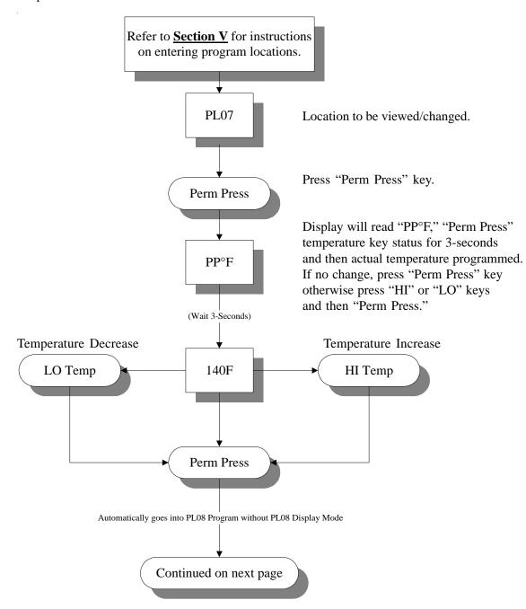
Summary: Perm press temperature is programmable from a minimum of  $100^{\circ}$  F to a maximum of  $160^{\circ}$  F in ten-degree increments or from a minimum of  $38^{\circ}$  C to a maximum of  $71^{\circ}$  C in five-degree increments.
