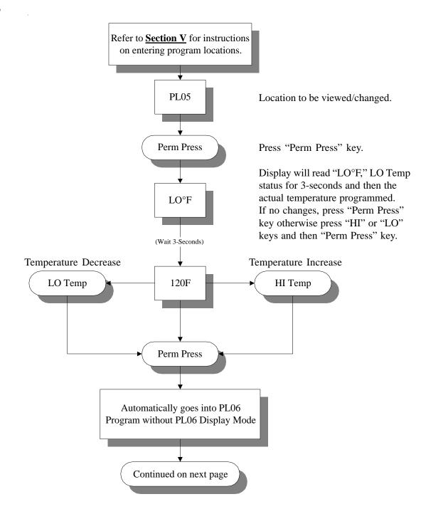
Summary: Low (LO) temperature is programmable from a minimum of  $100^{\circ}$  F to a maximum of  $160^{\circ}$  F in ten-degree increments or from a minimum of  $38^{\circ}$  C to a maximum of  $71^{\circ}$  C in five-degree increments.
