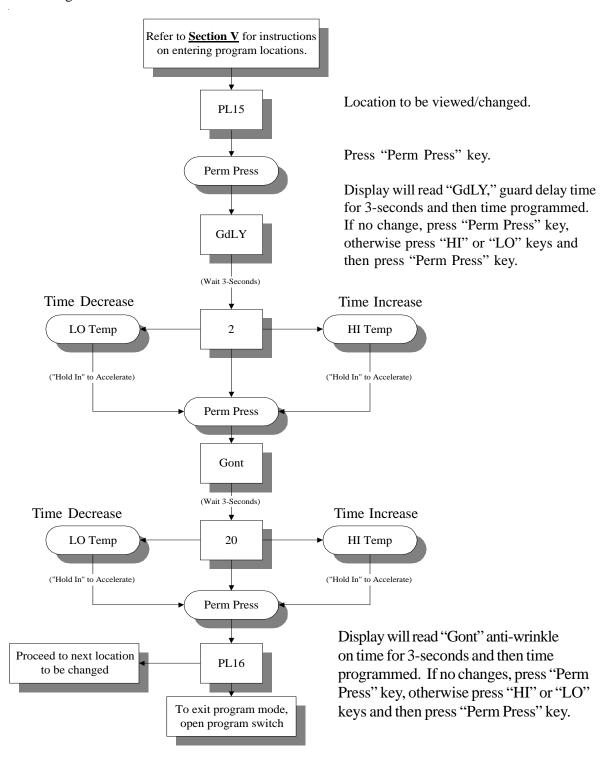
Summary: Guard delay time is programmable from 1 to 9 minutes. Guard on time is programmable from 1 to 99-seconds.
