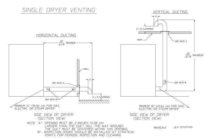
**IMPORTANT:** For extended ductwork runs, the cross section area of the duct can only be increased to an extent. When the ductwork approaches the maximum limits as noted in this manual, a professional heating, venting, and air conditioning (HVAC) firm *should be* consulted for proper venting information.
