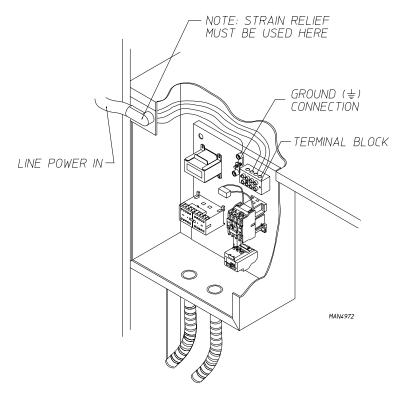
Providing local codes permit, power connections to the dryer can be made by the use of a flexible underwriters laboratory listed cord and pigtail (wire size **must conform** to rating of the dryer), or the dryer can be hard wired directly to the service breaker. In <u>ALL</u> cases, a strain relief **must be** used where the wires enter the dryer's electrical service (relay) box.
