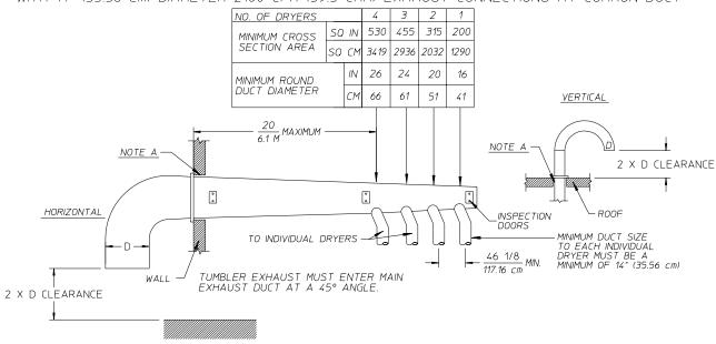
IMPORTANT: NO MORE THAN 4 DRYERS CAN BE CONNECTED TO ONE COMMON DUCT (VENT).
