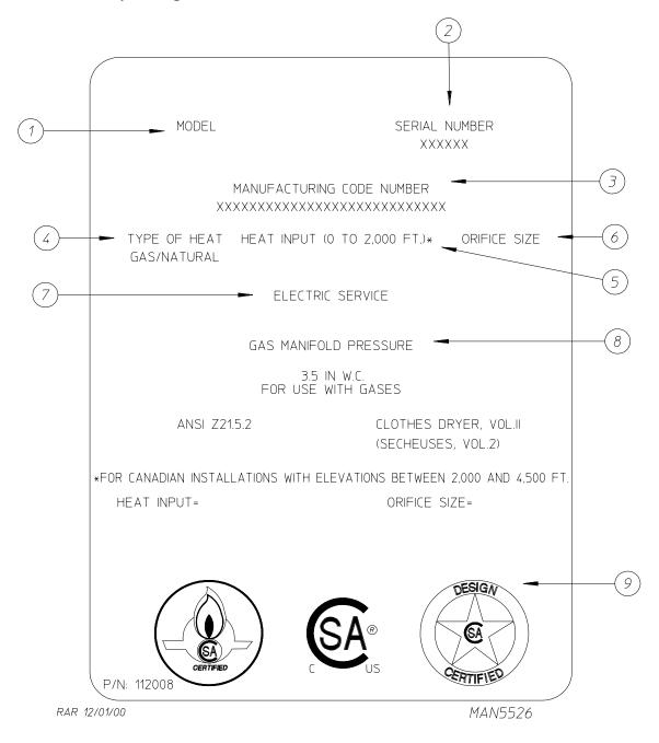
When contacting **American Dryer Corporation**, certain information is required to insure proper service/parts information from **ADC**. This information is on the data label located on the left side panel behind top/access control door. When contacting **ADC**, please have the <u>model number</u> and <u>serial number</u> available.
