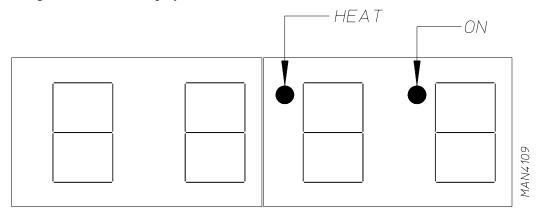
d. Verify that the motor(s), heat, and door indicator lights on the back side of the microprocessor controller (computer) board are lit. (Refer to the **illustration below**.)
