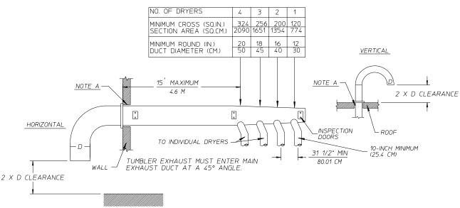
IMPORTANT: NO MORE THAN 4 DRYERS (8 TUMBLERS) CAN BE CONNECTED TO ONE COMMON DUCT ( VENT ).
