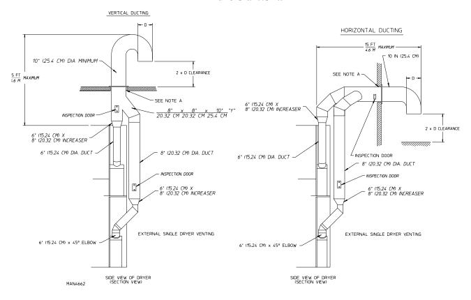
NOTE 'A': OPENING MUST BE TWO (2) INCHES (5,08 CM) LARGER THAN DUCT ( ALL THE WAY AROUND )
