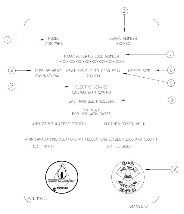
When contacting **American Dryer Corporation** certain information is required to insure proper service/parts information from **ADC**. This information is on the data label located on the inside of the control door. When contacting **American Dryer Corporation** please have the model number and serial number available.
