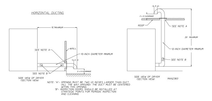
**IMPORTANT**: For extended duct work runs, the cross section area of the duct work can only be increased to an extent. When the duct work approaches the maximum limits noted in this manual, a professional heating venting air conditioning (HVAC) firm *should be* consulted for proper venting information.
