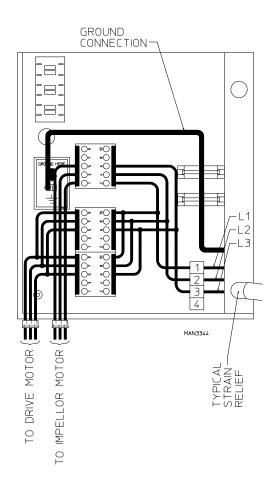
For gas dryers and steam dryers manufactured for operation at 3-phase  $(3\emptyset)$ , the electrical connections are made at the power distribution block located in the service box at the rear, upper left corner of the dryer. The ground connection is made to the copper lug also provided in this box. To gain access to the service box contactor, the service box cover **must be** removed.
