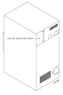
Actual electrical wire connections are made to the L1 and L2 terminals of the motor contactor located in the rear service box mentioned above. The ground connection is also made to the copper lug also provided in this box.
