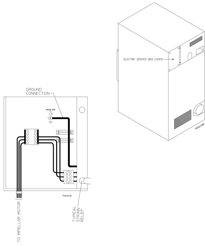
The electrical connections on <u>ALL</u> 3-phase  $(3\emptyset)$  gas dryers and steam dryers are made into the rear service box located at the upper left area of the dryer. Electrical connections for electrically heated dryers are made in the electric oven area located at the upper rear area of the dryer.
