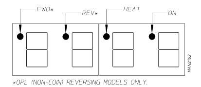
d. Verify that the motor(s) heat, and door indicator lights on the back side of the microprocessor (computer) board are lit. (Refer to the illustration below.)
