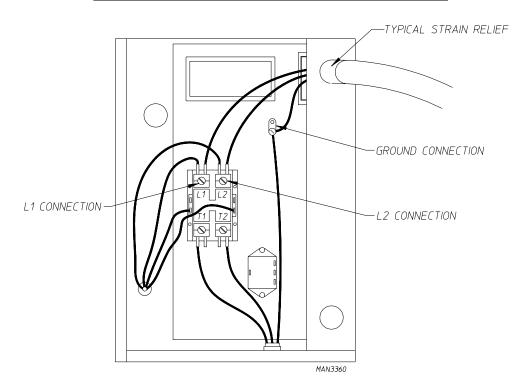
If local codes permit, power to the dryer can be made by the use of a flexible U.L. listed power cord/ pigtail (wire size **must conform** to rating of dryer), or the dryer can be hard wired directly to the service breaker panel. In both cases, a strain relief **must be** installed where the wiring enters the dryer.
